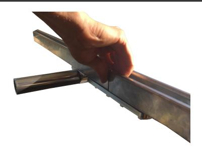
**Step 19:** Snug the two mending plate secure bolts connected to the extension fence strut rail from Step 18.
