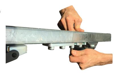
**Step 22:** Firmly tighten the elevation jam nut down to the stand post to lock in the height of the extension fence strut rail. Tools Needed: 10"+ crescent wrench.
