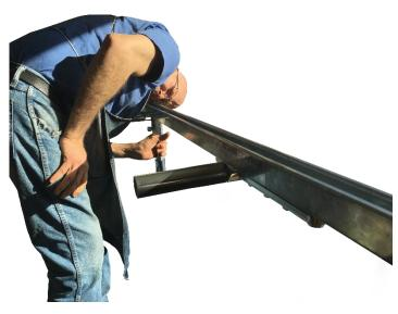
**Step 21:** Firmly tighten the mending plate secure bolts connected to the extension fence strut rail. Tools Needed: 3/8" Allen wrench.
