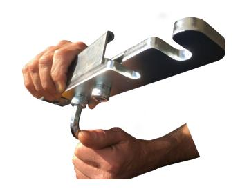
**Step 13:** Place the remaining mending plate nut over the 1<sup>st</sup> and 2<sup>nd</sup> holes (counting from the saw side). Just barely thread in two mending plate secure bolts from the bottom while keeping the mending plate nut relatively centered and back from the edge by 1/16".
