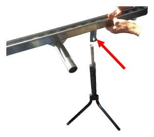
**Step 15:** Place the extension fence strut rail onto the stand post by inserting the elevation rod into the stand hex mount.
