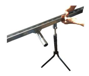
**Step 16:** Loosen the elevation jam nut from the stand post. Tools Needed: 10"+ crescent wrench.
