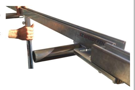
Step 18: Slide the two mending plate secure bolts connected to the extension fence strut rail into the open slots on the mending plate. You may have to loosen the two mending plate secure bolts in order to slide them into the mending plate.
