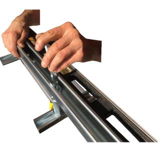
**Step 28:** Check the fence strut rail to see if there is a 1/16" clearance between the fence strut rail and straightedge. If not, adjust the fence strut rail.
