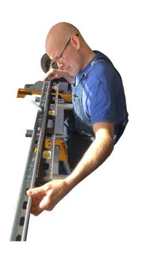
**Step 29:** Firmly tighten both fence secure bolts securing the fence strut rail to the elevation bolts. Tools Needed: 3/8" Allen wrench.
