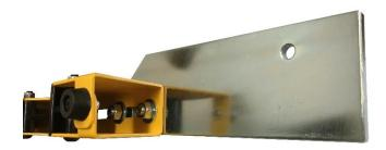
Step 5: Slide one of the front plates so that the bolts are hitting the front edge of the slot, and the outside edge of the plate is flush with the outside edge of the mounting bracket. Tighten the plate mounting bolts. Tools Needed: 3/16" Allen wrench and 1/2" wrench.
