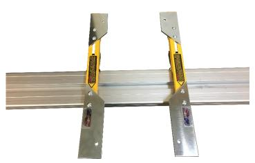
Step 3: Place the back right plate and back left plate onto their mounting brackets. Use two plate mounting bolts, two washers, and two nuts to secure each plate to the mounting bracket. Hand tighten each nut.
