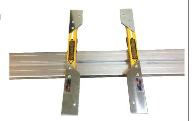
**Step 13:** Place your saw onto the assembly. Push a saw mounting bolt through each of the mounting holes on your saw and through the hole on the respective plate.
