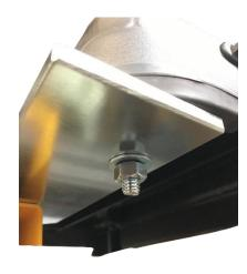
**Step 15:** Tighten each of the nuts. Tools Needed: 3/16" Allen wrench and 1/2" wrench.
