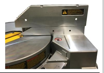
**Step 5:** Bring the saw down to the lowest position.
