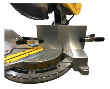
**Step 8:** Scribe both of the drill locations by tracing the edge of both saw fence holes. Access these holes from the back of the saw fence.
