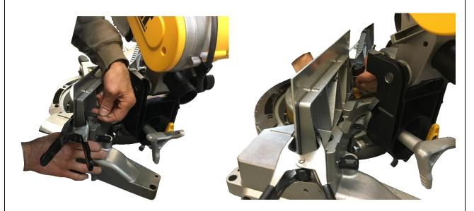
**Step 9:** Unclamp the zero clearance fence from the saw fence.
